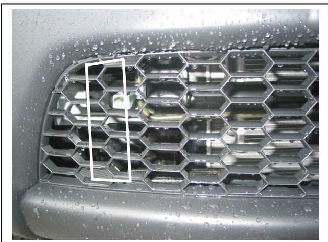
Figure 3: Area to be trimmed on lower centre grille.
