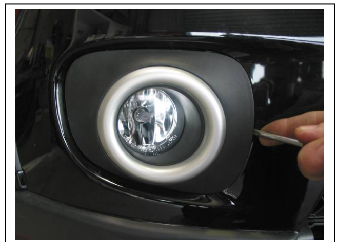
Figure 8: Use a flat bladed screw driver to carefully remove fog light covers. Fog light model shown
